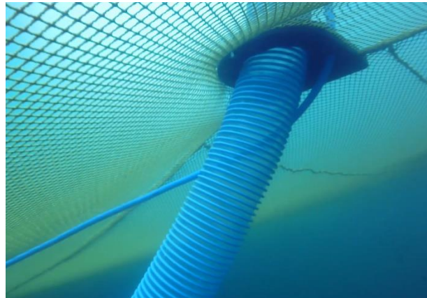
Figur 9 LiftUp slange under nottak under drift
