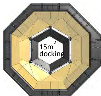
Figure 5a-c, iFarm floater and net docking opening, Docking mounted reducing the opening from 7 to 4m, iFarm floater, bottom ring, and upper part of net docking (net roof missing).
