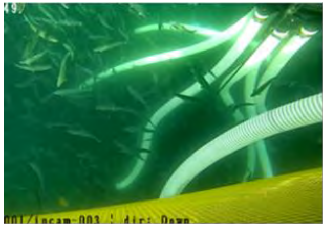
Figure 9b, iFarm feeding system when mounted in a snorkel without iFarm house.
