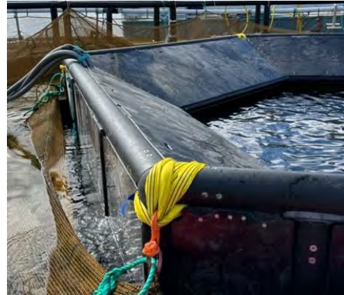
Figure 5d, Docking being lifted in the cage by a farm boat. Figure 5e, Docking mounted with 6x 9T rope shackles.
