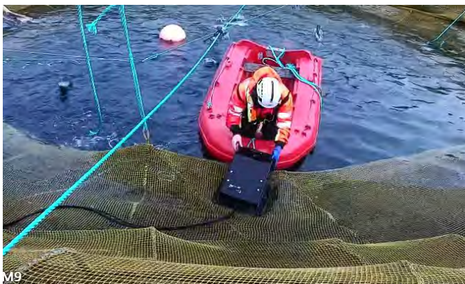
Figure 6a IP camera box mounted on the net docking, which is later moved to docking when this is installed.
