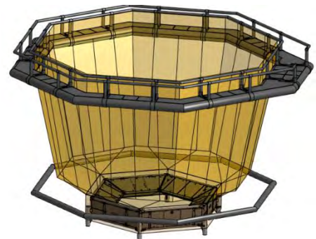
Figure 5a-c, iFarm floater and net docking opening, Docking mounted reducing the opening from 7 to 4m, iFarm floater, bottom ring, and upper part of net docking (net roof missing).
