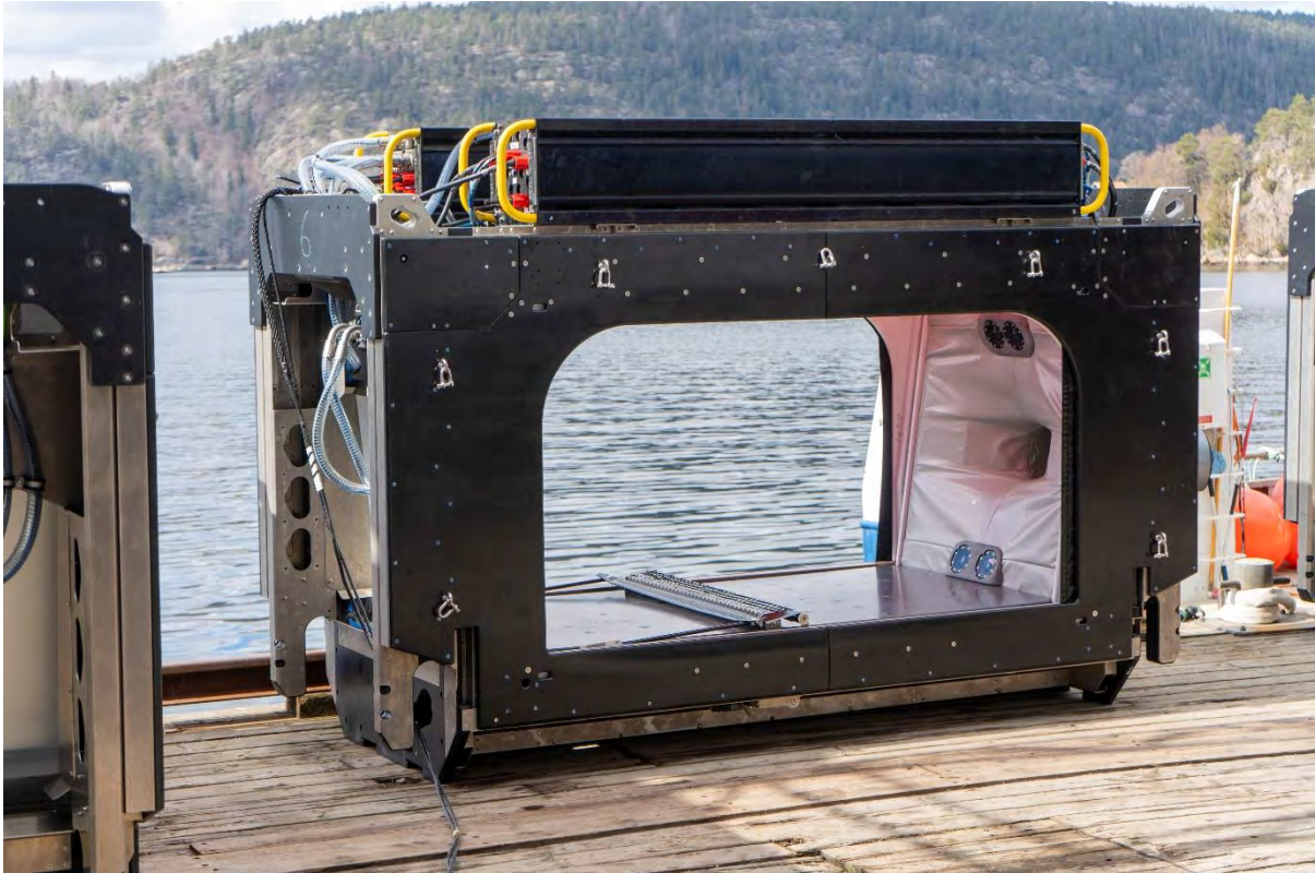
Figure 11 3 rd generation sorter opening with smooth opening for guiding fish into the transportation channel.
