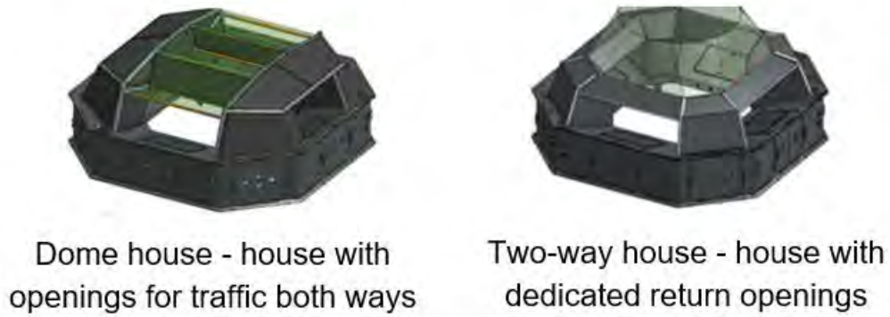
Figure 12: Illustration of the phase 2 Dome house with openings for swimming in both directions to the left and the phase 2 Two-way house with dedicated return openings to the right.
