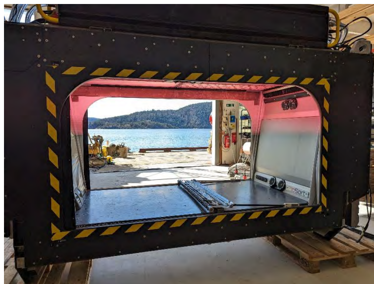
Figure 31: iFarm sensor and sorting opening unit on land. Foldable sorting walls lay in resting position in the middle of the sensor.
