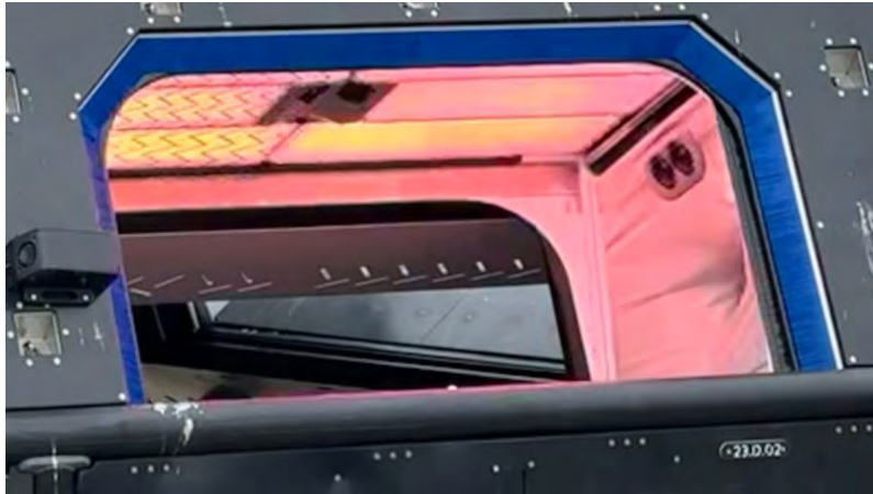
Figure 22: The iFarm sensor and sorter opening in phase 4. Cameras are placed in the top and bottom of the sensor sides and in the sensor ceiling.
