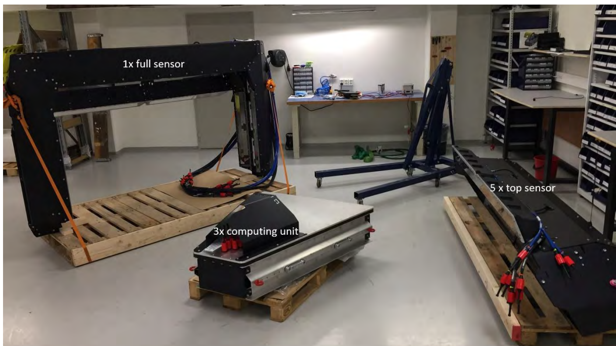
The sensor arrangements shipment to be assembled with the Dome and the Saddle housing consisted of 1 full sensor, 5 top sensors, and 3 computing units
